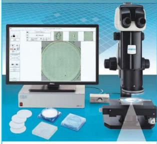
Microscopic analysis of residue particles on filter membranes
