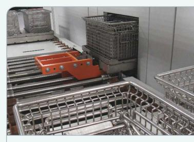
:: The Roll system was custom built with adapter frames to accommodate the use of baskets from Precision Plus' previous cleaning unit. Two baskets can be used at the same time, doubling throughput.
