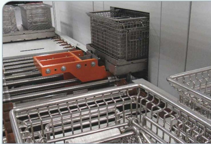
∴ The Roll system was custom built with adapter frames to accommodate the use of baskets from Precision Plus' previous cleaning unit. Two baskets can be used at the same time, doubling throughput.
