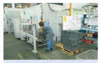
The new cleaning system makes it possible to comply with very high standards for the removal of particulate matter and films.
