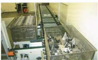
The cleaning baskets are transported through the machines and on to the subsequent areas on the first-in-first-out principle.
