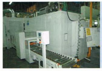
In order to prevent the parts being recontaminated with environmental dirt after cleaning, the unloading area is enclosed in a tunnel. Excess pressure from the clean room helps to ensure that the clean parts do not become dirty again.
