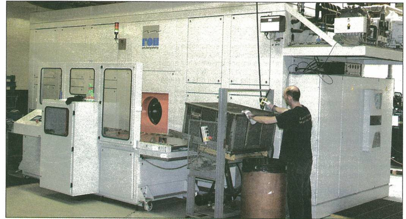
UniMetal recently made a major financial investment in a new, state-of-the-art, automated Roll parts vacuum ultrasonic cleaning machine, seen here. The Roll machine, being operated above by Keith Gallion, is more efficient and more environmentally friendly. Contributed.
