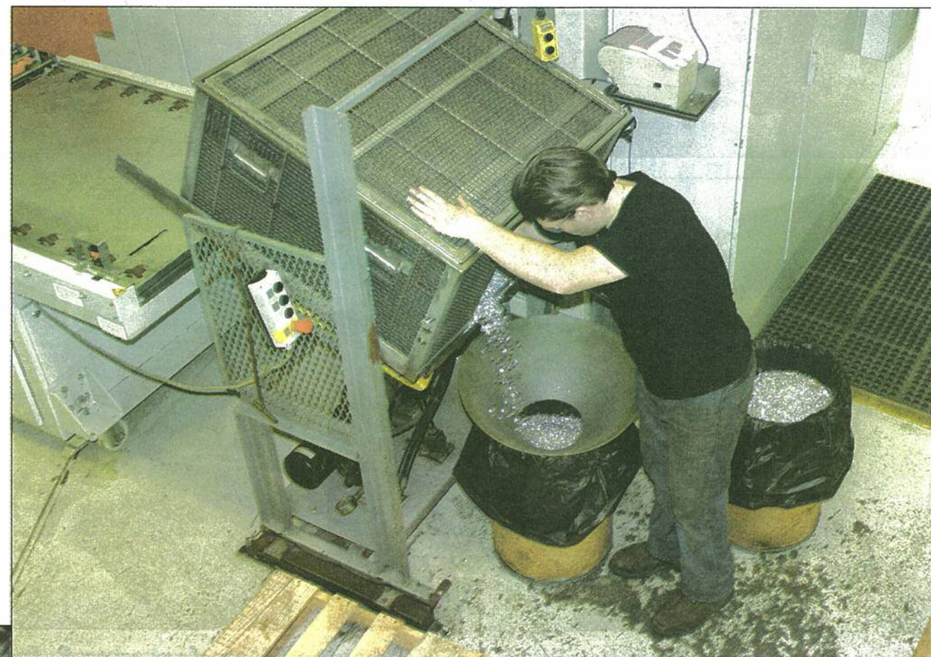
Above: UniMetal's Tony Bonatsos empties cleaned parts from the company's new Roll parts vacuum ultrasonic cleaning machine back into a customer's container, which is lined with a plastic bag to maintain cleanliness. Contributed.
