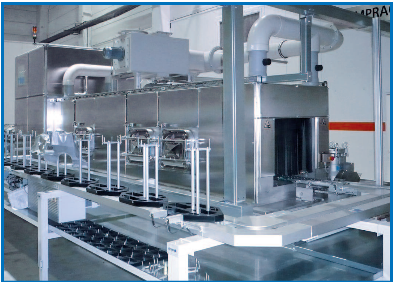
Pass-through spray facility with part transport device
